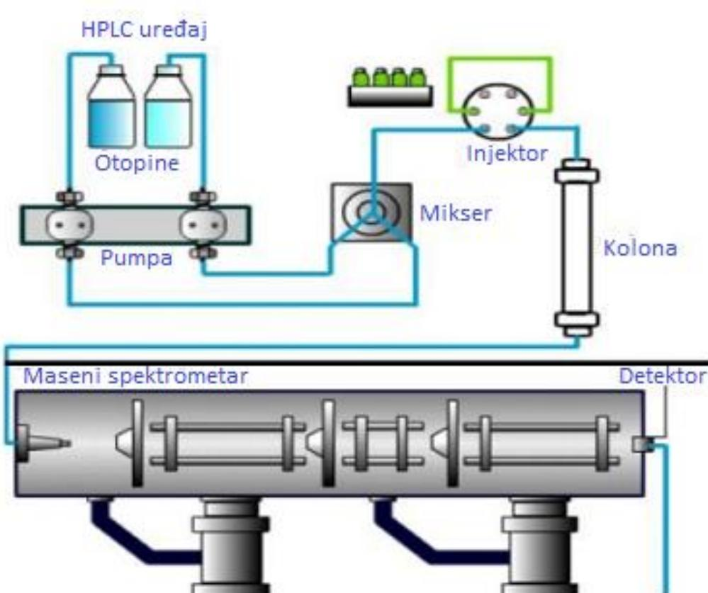
Slika 12. Shematski prikaz LC-MS (preuzeto s [www.slideshare.net](http://www.slideshare.net)).
