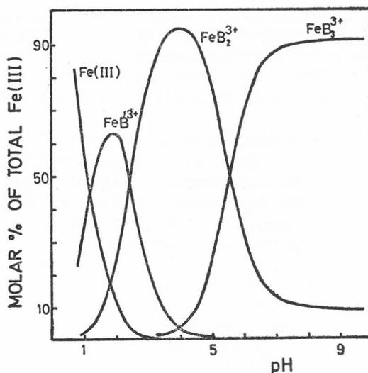
Figure 4. (B) Distribution of different iron(III) species as a function of pH of the solution. Conditions of (A) and (B) :  $5 \times 10^{-4}$  M  $\text{FeCl}_3$ ,  $10^{-2}$  M betaine hydroxamic acid. 1.0 M ionic strength (NaCl), 25 °C.
