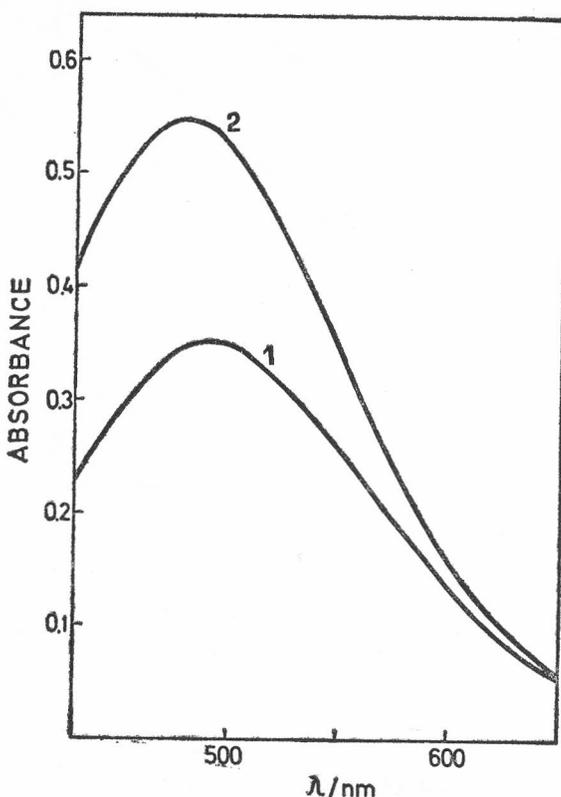
Figure 1. Visible spectrum of monoglyciniumhydroxamatoiron(III) (1) and monobetainehydroxamatoiron(III) (2) complex. Conditions: 0.15 M  $\text{FeCl}_3$ ,  $5 \times 10^{-4}$  M hydroxamic acid, 0.1 M HCl, 1.0 M ionic strength (NaCl), 25°C. The spectra are taken against 0.15 M  $\text{FeCl}_3$  in 0.1 M HCl as a blank.
