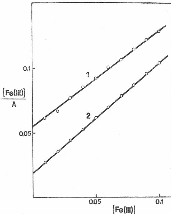
Figure 2. The ratio of the total iron(III) concentration to the absorbance vs the total iron(III) concentration at 500 nm. Conditions:  $5 \times 10^{-4}$  M glycinium hydroxamic acid (1) or betaine hydroxamic acid (2), 1.0 M ionic strength (NaCl), 0.1 M HCl, 25 °C.
