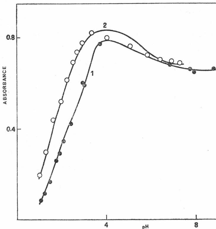
Figure 3. Dependence of the absorbance at 500 nm on pH of solution, Conditions:  $5 \times 10^{-4}$  M  $\text{FeCl}_3$ ,  $1 \times 10^{-2}$  M glycinium hydroxamic acid (1) or betaine hydroxamic acid (2), 1.0 M ionic strength (NaCl), 25 °C.
