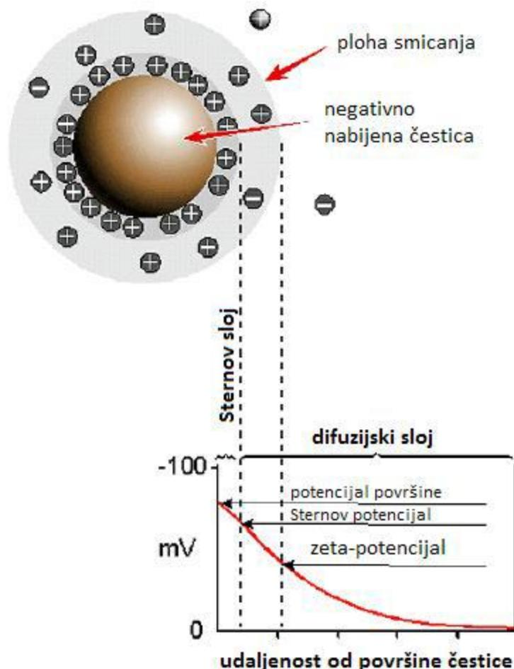
Slika 6. Shematski prikaz zeta potencijala (preuzeto s [www.malvernpanalytical.com](http://www.malvernpanalytical.com))
