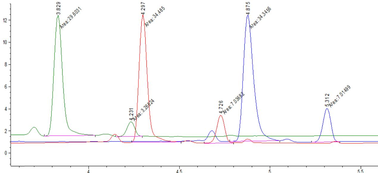
Slika 13. Elektroferogram standardnih otopina ribocikliba (50  $\mu\text{g}/\text{ml}$ ) i unutarnjeg standarda diazepama (50  $\mu\text{g}/\text{ml}$ )
