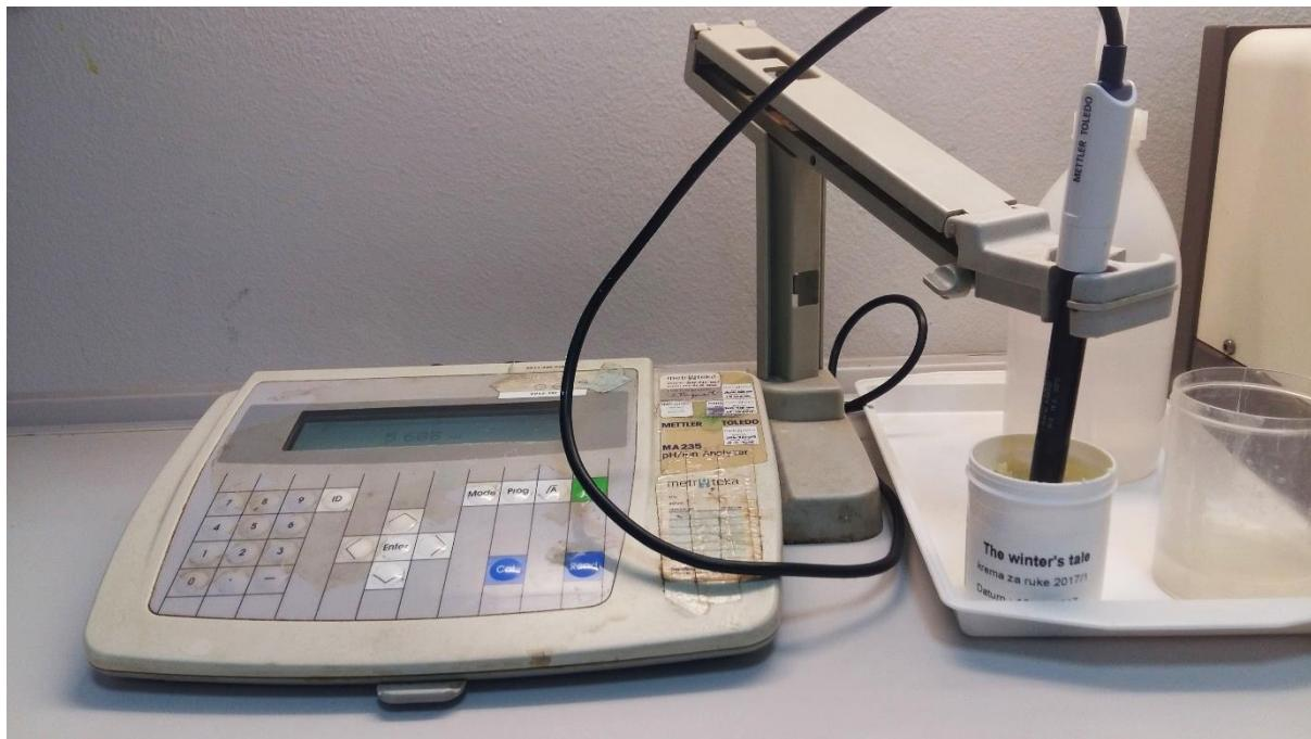
Slika 17: pH metar Mettler Toledo MA 235
