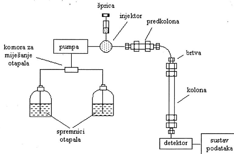
Slika 10: Shematski prikaz HPLC kromatografa ([http://free-zg.t-com.hr/Svetlana\\_Luterotti/09/091/09131.htm](http://free-zg.t-com.hr/Svetlana_Luterotti/09/091/09131.htm))
