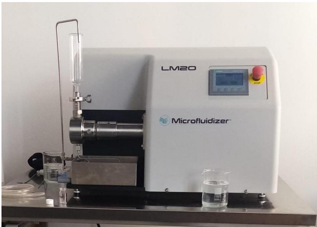
Slika 4. Mikrofluidizator model LM20 Microfluidizer®
