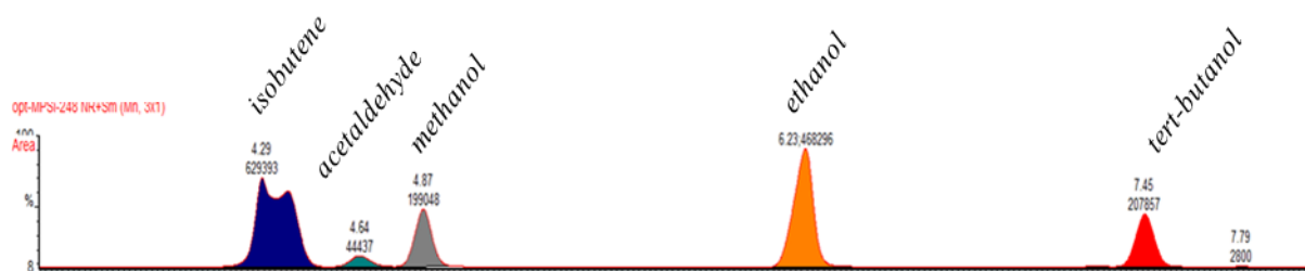
Figure 9. TD-GC-FID chromatogram of the toluene solution at the lower trap temperature (4 °C).
