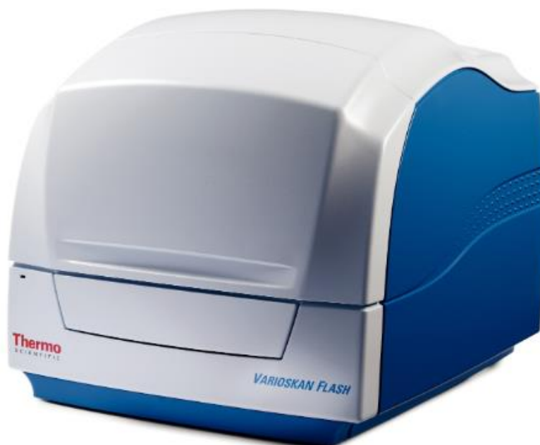
Figure 19. Varioskan Flash spectral scanning multimode reader (Thermo Fischer Scientific Inc, USA) used in this study to measure luminescence in cell viability assays ( http://www.thermoscientific.com/en/product/varioskan-flash-multimode-reader.html ).
