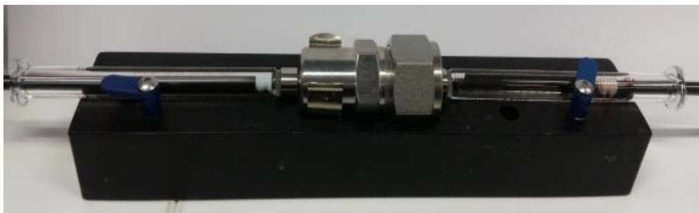
Figure 17. Avanti Mini-Extruder used for production of Ps with main size around 200 nm ( http://www.sapphirebioscience.com ).
