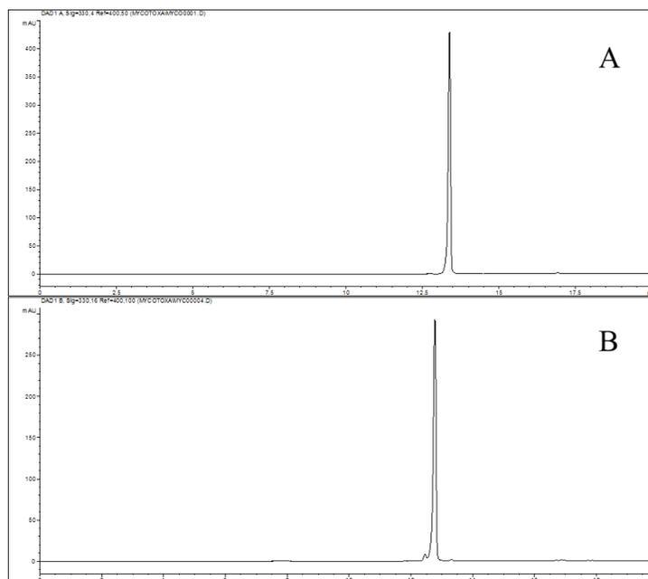
**Slika 5.** UV/Vis kromatogram (A) sterigmatocistina i (B) 5-metoksisterigmatocistina. *Uvjeti analize: Symmetry kolona C18 4,6x150mm, 3,5  $\mu$ m, temperatura kolone 35  $^{\circ}$ C, mobilna faza A: metanol, B: voda; brzina protoka 1,0 ml/min; gradijent: 0-6 min 48% B, 6-14 min 48  $\rightarrow$  10% B, 14-25 min 10% B, 25-26 min 10  $\rightarrow$  48% B, 26-40 min 48% B. Valna duljina detekcije 330 nm.*
