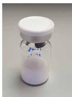
Figure 1. Azelaic acid nanocrystals lyophilizate.
