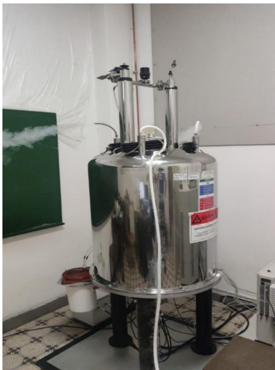
Slika 4: NMR instrument Varian INOVA 400
