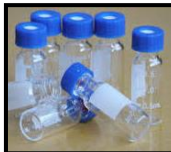
Slika 9: HPLC staklene vialice (preuzeto s https://www.indiamart.com/proddetail/hplc-vials-7616795988.html )
