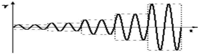
Figure 12. Schematic representation of strain sweep test (reprinted from (105)).
