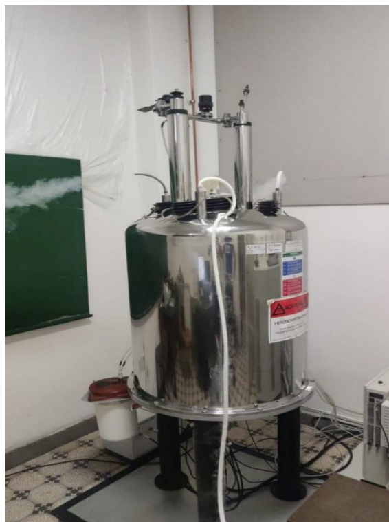
Slika 4: NMR instrument Varian INOVA 400
