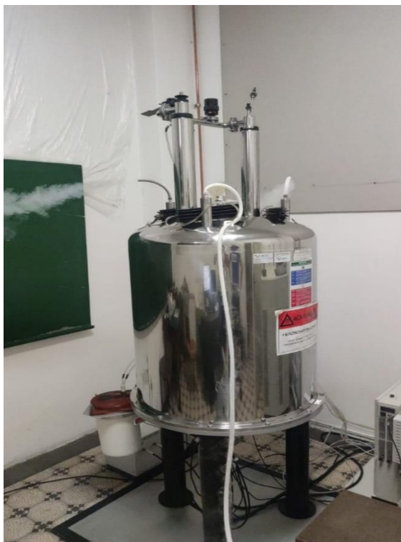
Slika 4: NMR instrument Varian INOVA 400
