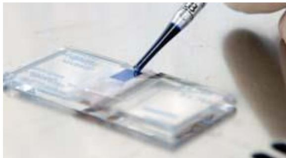
Slika 6. Prikaz stavljanja uzorka automatskom pipetom (preuzeto prema: <http://www.sigmaldrich.com/technical-documents/protocols/biology/cell-quantification.html>).
