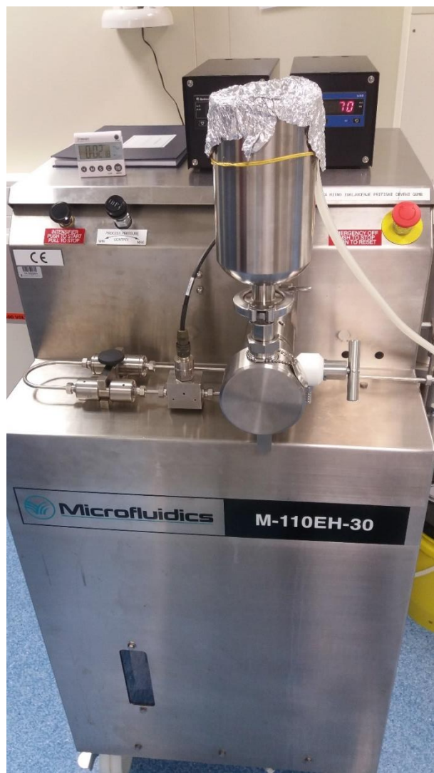
Slika 4. Mikrofluidizator (Model M-110EH-30 Microfluidizer, Microfluidics, Newton MA, SAD), PLIVA Hrvatska d.o.o..
